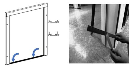
3. Installing the lower guide profile
